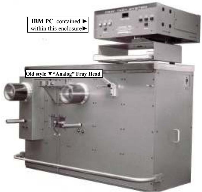
In 2000, Javatec redesigned the Fray Detector Head assembly in the Fray Tester that was originally conceived and manufactured in 1987 from an Analog device, using Photo Diodes and a significant amount of external circuitry to a State-of-the-Art Digital
