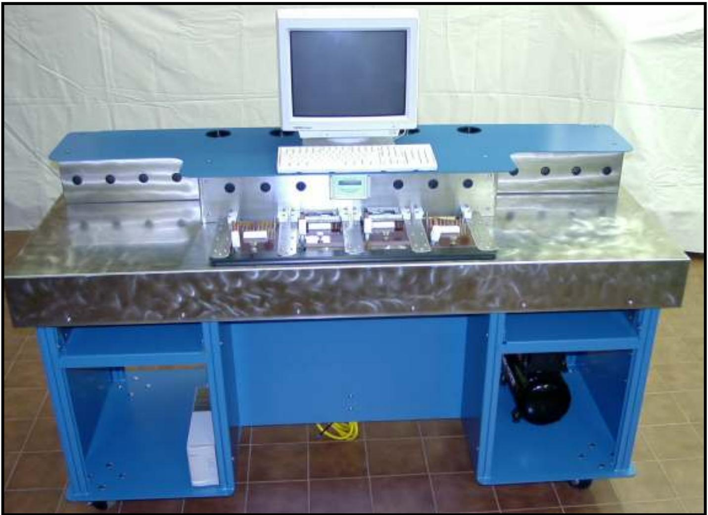
The above System was designed to simultaneously test 4 Printed Circuit Boards, each containing a very low (0 to  $\pm 1$  Inch of water) Differential Pressure Transducer. This System would generate and monitor pressures that would range from 0.0000 to 0.9999 inch of water. There was a computer controlled PID loop that would read the Supply Pressure and then control a Stepper Motor (Micro-steps) that would adjust a precision mechanical Needle Valve to obtain the desired Test Pressure.
