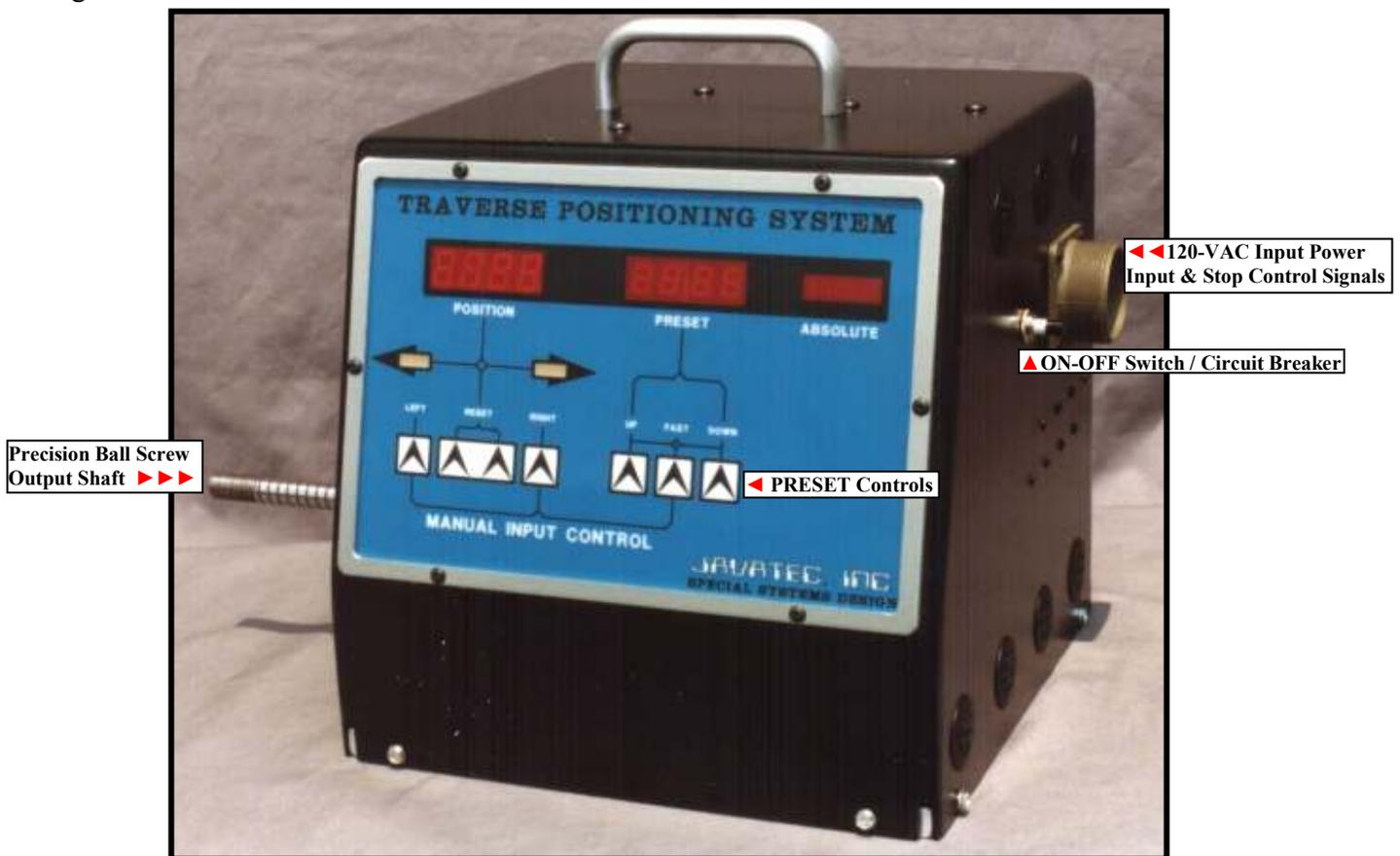
All of the Control Electronics, Stepper Motor, Mechanical Drive Components and Power Supplies were contained in a 10x10x10 Enclosure as shown above and the "Heart of the system was a Microprocessor.
